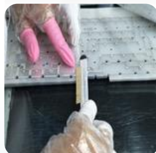
Paste Conductive Tape
