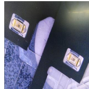
LED inspection by CCD
